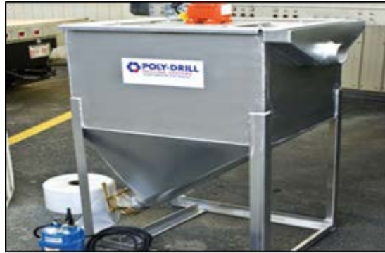
Figure 12-8 – Poly Drill Filter Box Used for Solids Removal in Drilling Applications
