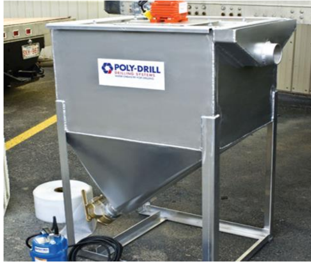
Figure 11-4 - Polydrill Filter Box used for Solids Removal in Drilling Applications
