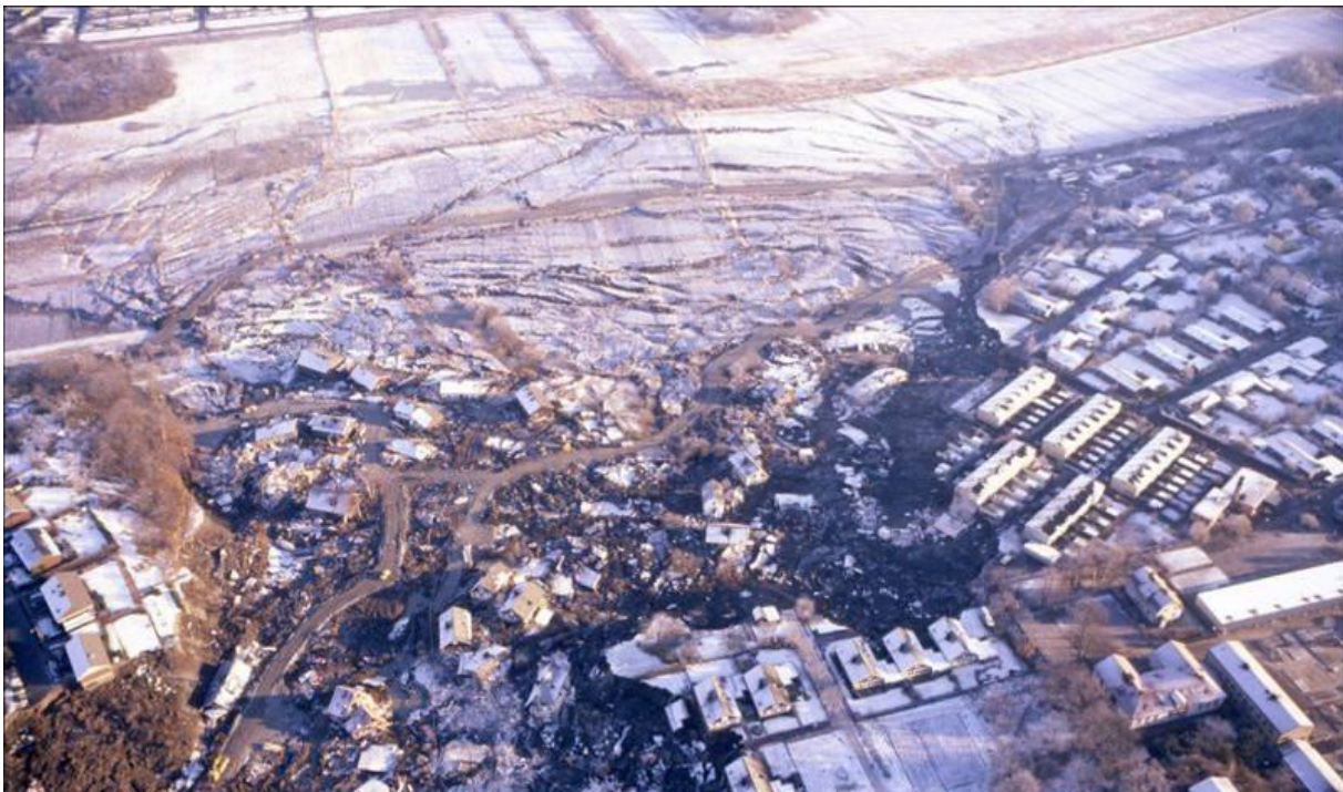
Figure 2-1. Aerial photograph of the Tuve slide in Gothenburg 1977 with East in the top. The slide started in the middle of the photo and moved beyond the Kville Creek (top). Copyright Gothenburg Museum of Natural History, Bernander et al (2016).
