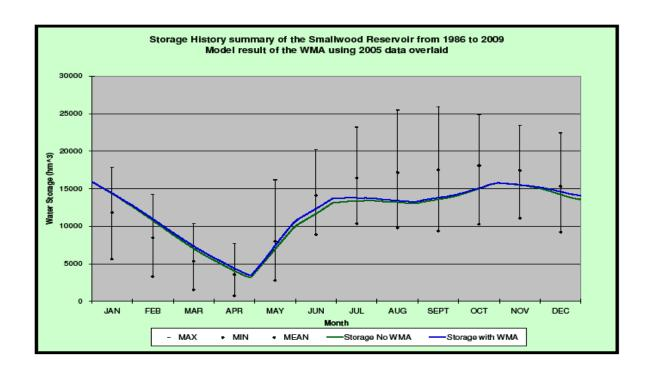
As shown in the diagram, the difference is minimal and would not have an adverse effect on the reservoir.
