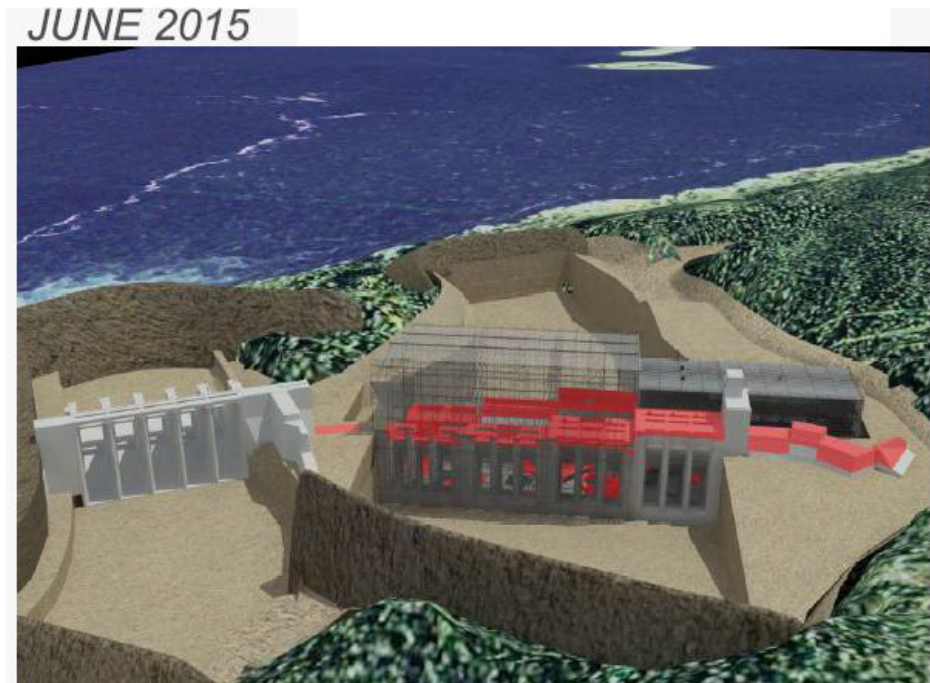
Figure 9: Astaldi as-planned status of the civil structures by June 2015 – CH0007 Construction visualization with Astaldi bid (Upstream view). Note the intended status, particularly in the intake (foreground, mid-right side of photo), as well as the powerhouse building erected over the South Service Bay and Unit 1, while the ICS remains in place over units 2, 3, and 4, as well as the North Service Bay.
