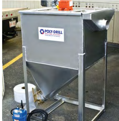
Figure 5-3: Poly Drill Filter Box used for solids removal in drilling applications
