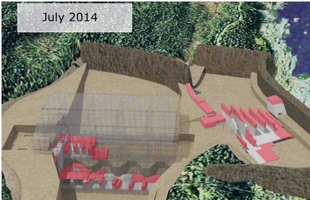
Figure 16: Intake, Powerhouse and Spillway civil works mid-2014
