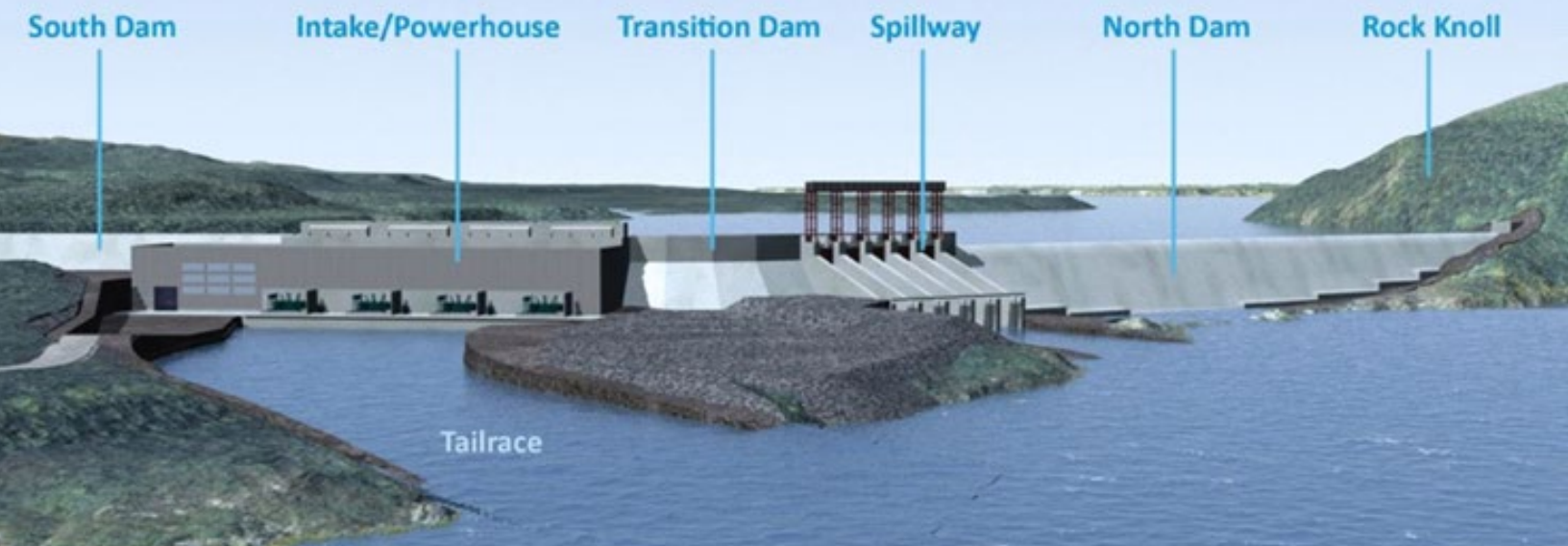
Figure showing the Muskrat Falls Generating Facility
