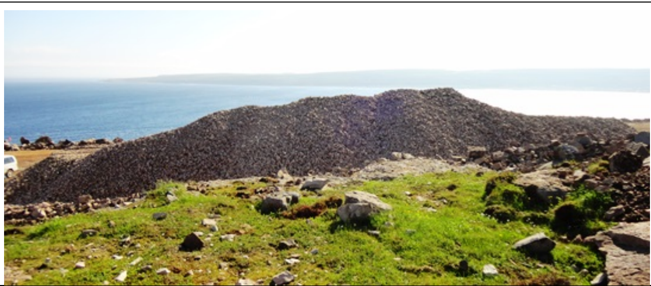
Photo 4.3: Forteau quarry. Stockpile of processed rockfill. (July 15, 2014)
