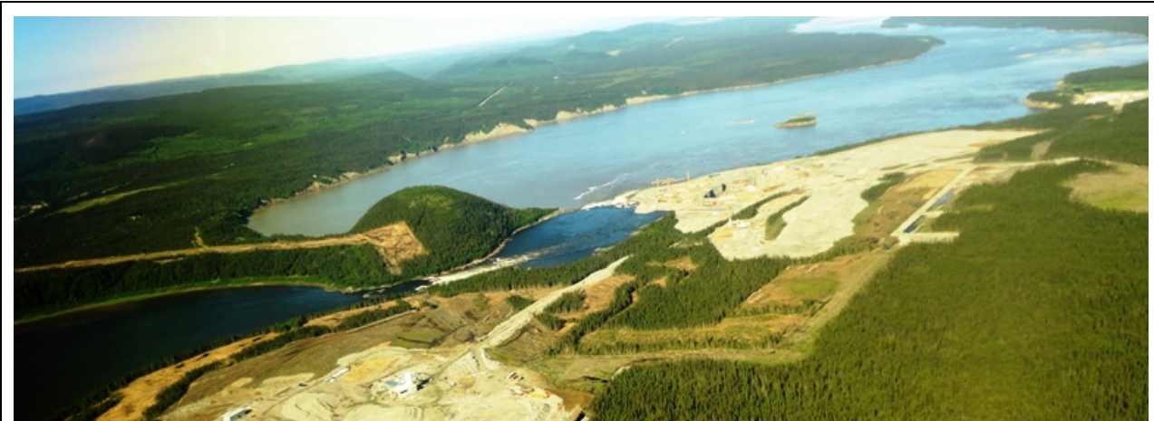
Photo 6.1: Panoramic view of the Muskrat Falls site looking towards downstream (July 18, 2014). The powerhouse/spillway site is visible on the upper right side of the photo. Transmission line clearing on the North Spur and reservoir clearing upstream of the falls are visible in the left side of the photograph.
