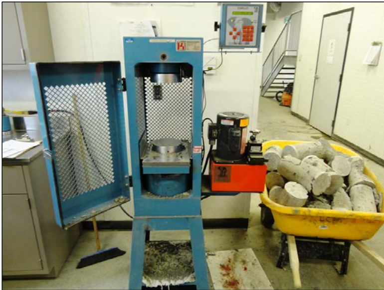
Photo 6.4: Site laboratory , unconfined compressive strength testing of concrete cylinders.
