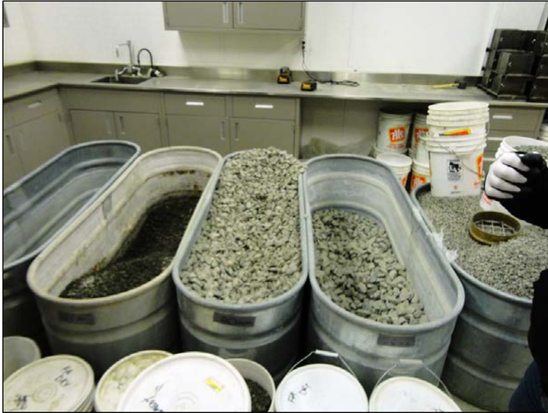
Photo 6.3: Site laboratory; graded aggregates for concrete mix design. (November 25, 2016)
