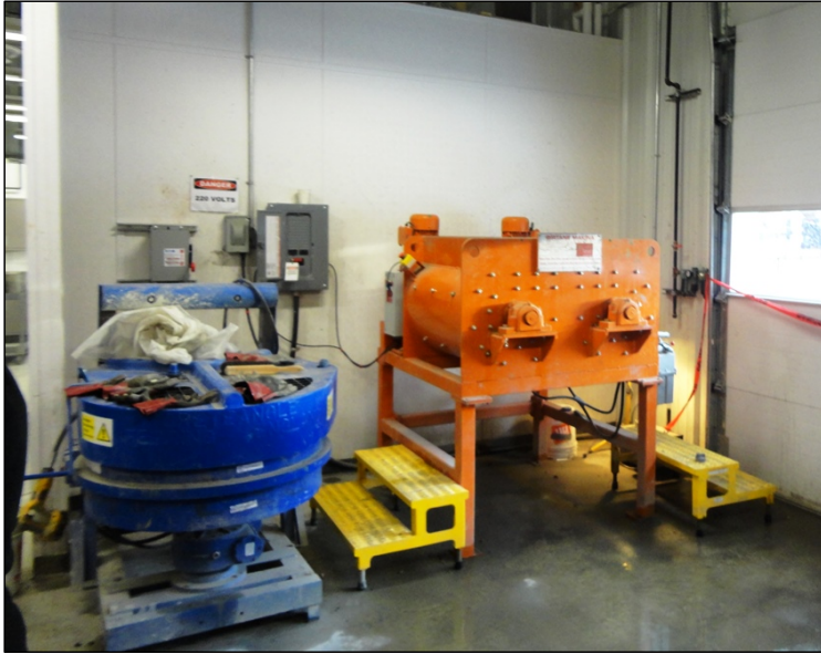
Photo 6.1 Site laboratory; mixer for concrete mix design. (November 25, 2014)
