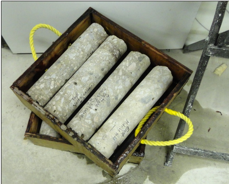
Photo 6.5: Drilled concrete cores from the field
