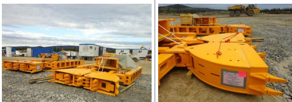
Photo 3.17: New clamshell buckets, to be used for deeper sections of the cut-off wall.
