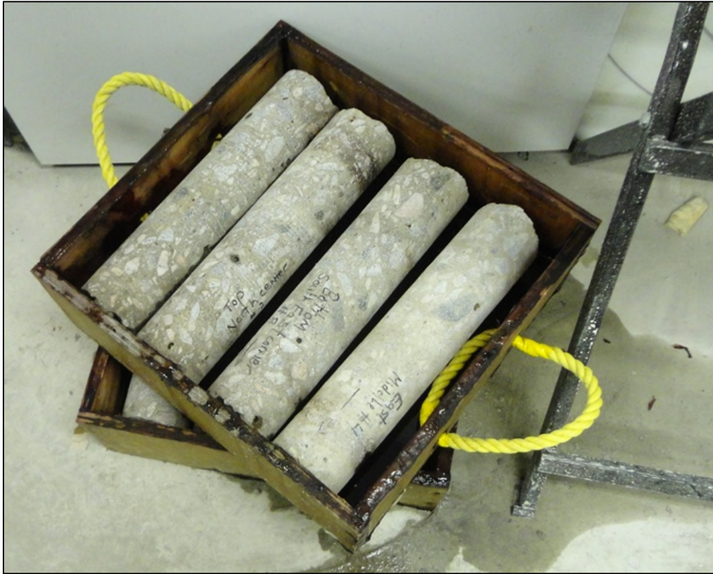
Photo 6.5: Drilled concrete cores from the field. (November 25, 2016)
