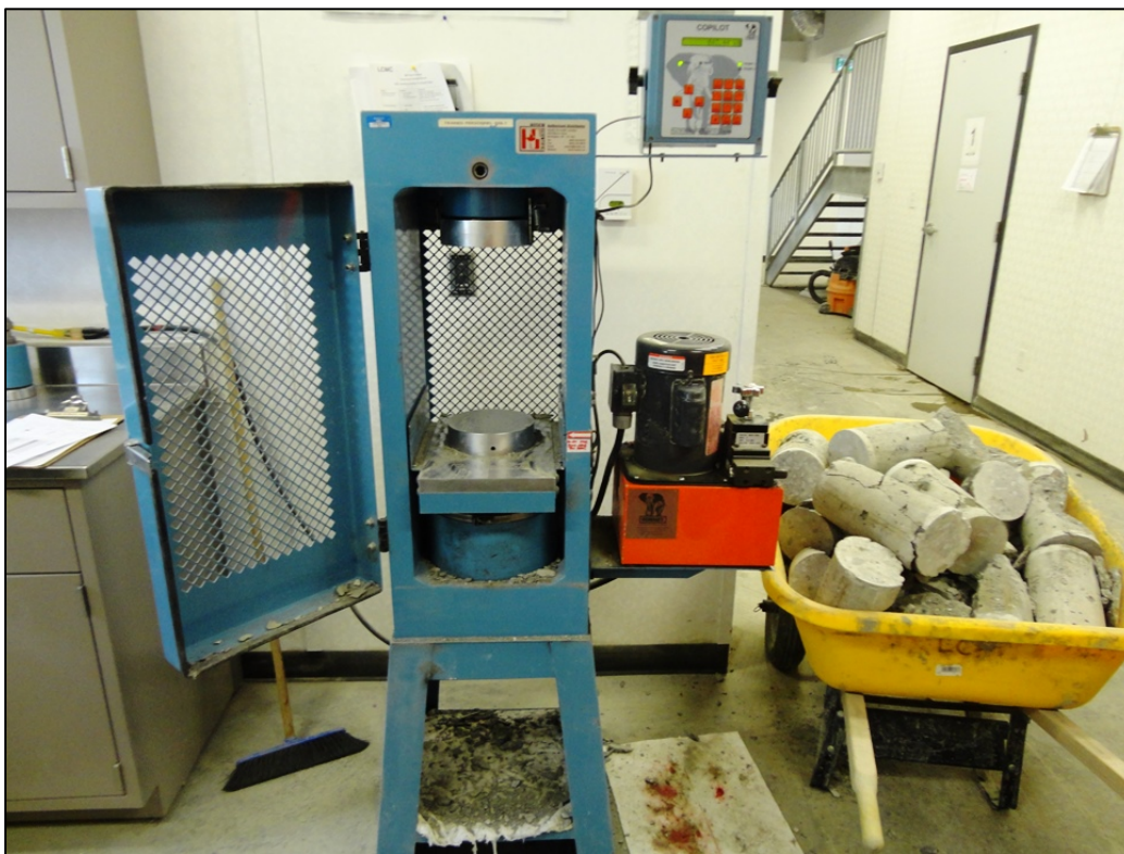
Photo 6.4: Site laboratory , unconfined compressive strength testing of concrete cylinders. (November 25, 2016)
