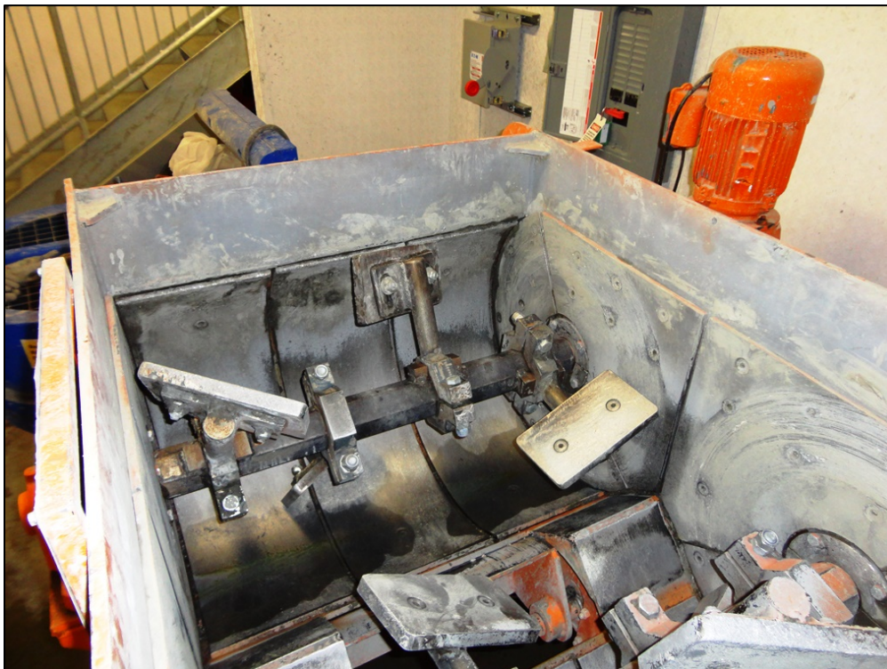
Photo 6.2: Site laboratory; mixer for concrete mix design. (November 25, 2014)
