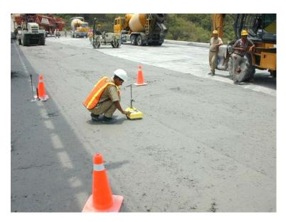
Figure 12: RCC Density Measurement (Porce II Dam, Colombia)
