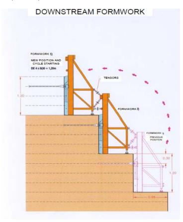
Figure 33: Dragados' Proprietary Formwork System for RCC Construction
