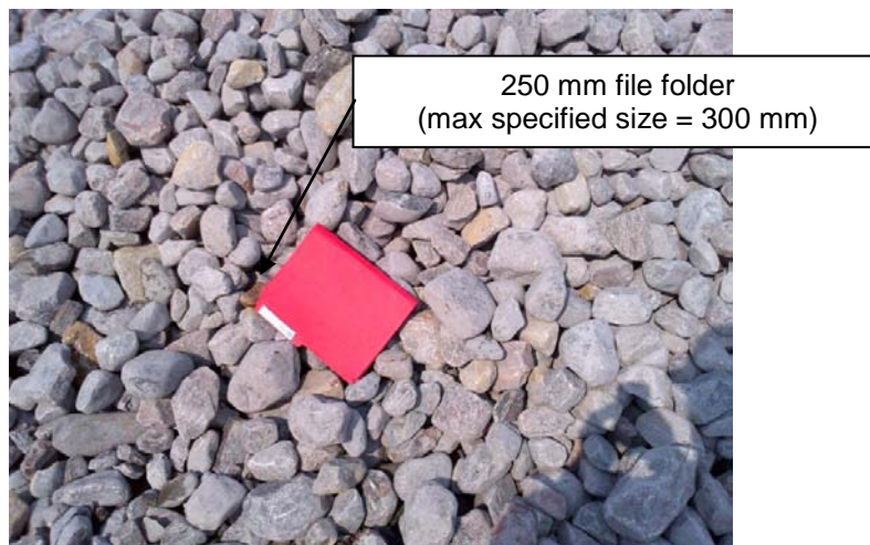
Figure 3-2: View of one of the Oversized Waste Stockpiles
