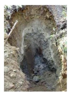
North and East coordinates obtained using Garmin Etrex Legend Cx GPS. Water entering test pit at 3.5 meter mark, slow trickle.
