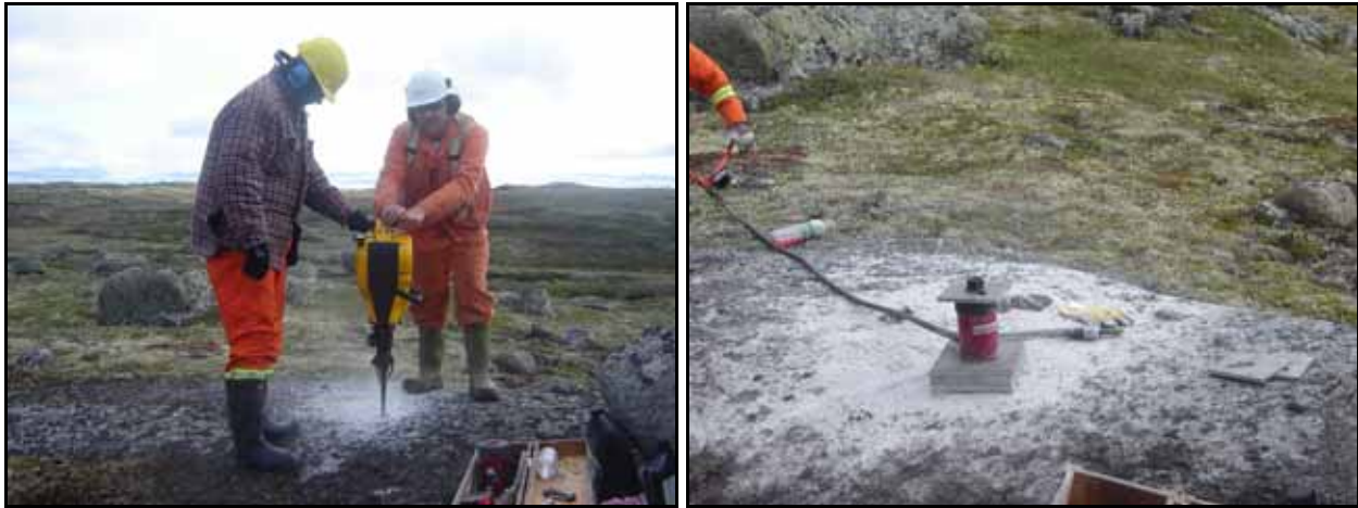
Photo 5 and 6: Pionjar drilling a test hole and the hydraulic jack conducting the test
