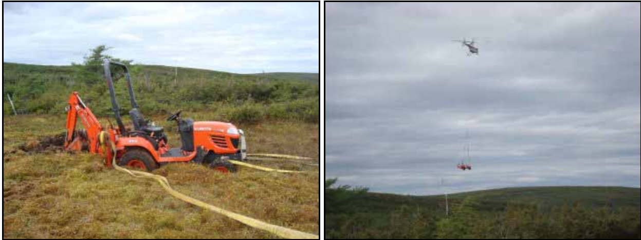
Photo 1 and 2: BX-24 Kabota with associated sling equipment and being slung via helicopter.
