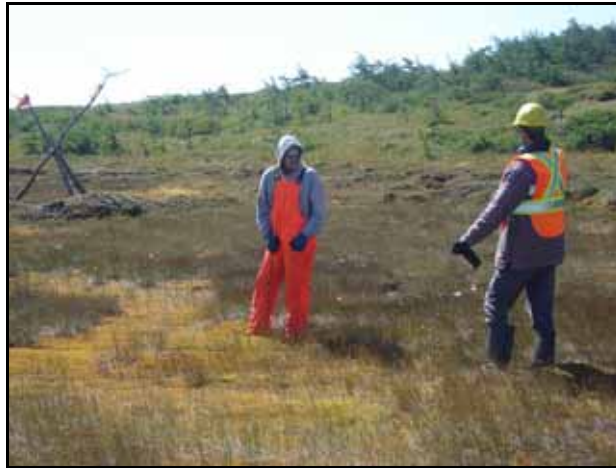
Photo 7: Field personnel probing boggy terrain with reinforcing bar.
