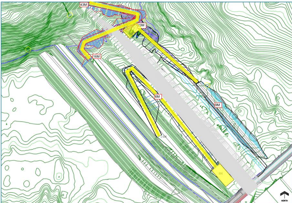
Crane Access Pads and Ramps, Upstream and Downstream of the North Dam
