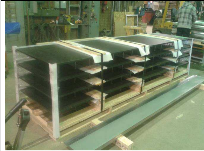
Picture No : 01 Brief Description : Packaging of side lining plates after paint work (06 Mar 2014)
