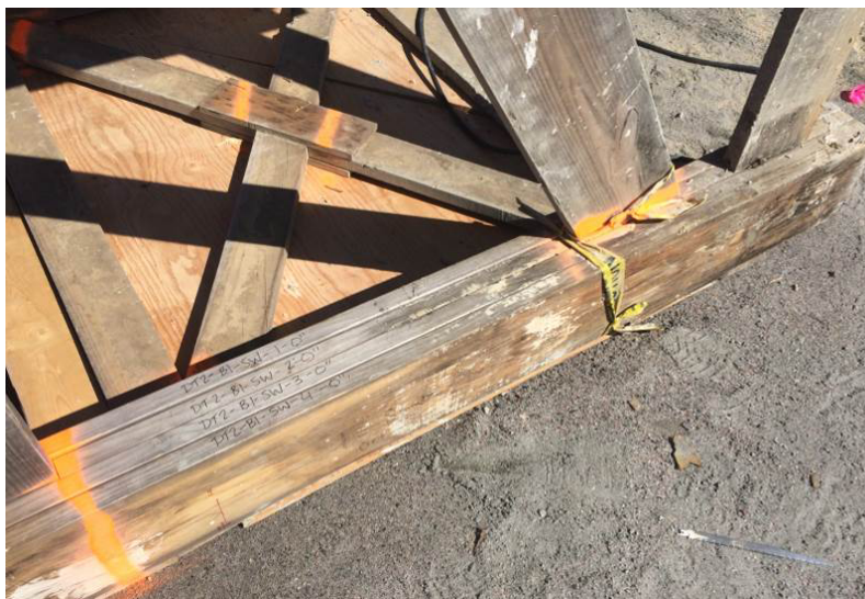
Figure 39: SW Tower Leg of B2 recovered from DT2, submitted for testing
