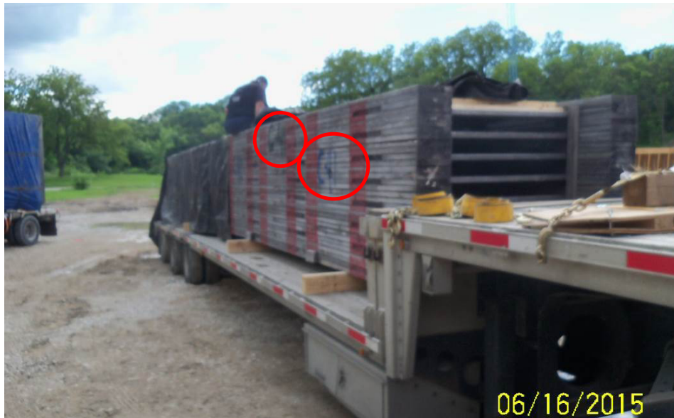
Figure 23: Falsework with multiple color markings "C41" at CEI's facility
