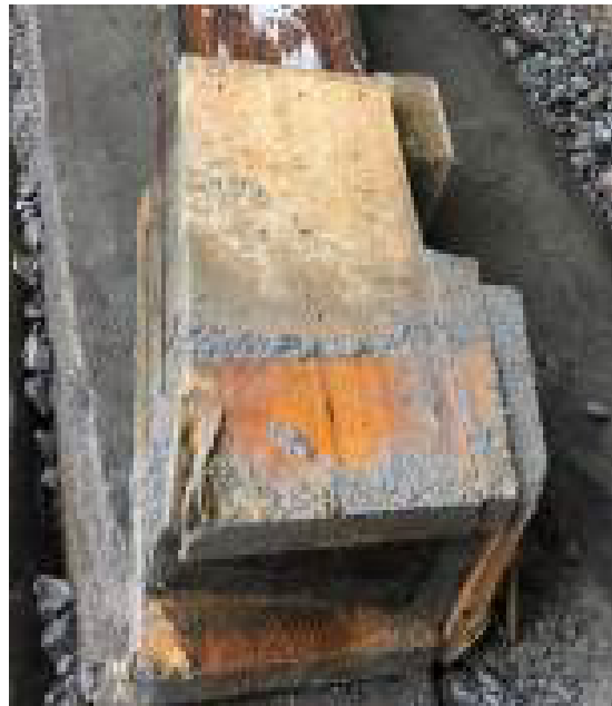
Figure 61: Alternate grout form at base of falsework tower leg. Recovered from Row C towers DT2
