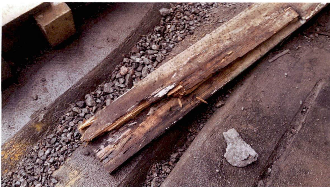
Unit 2 - Shoring tower rotten lumber
