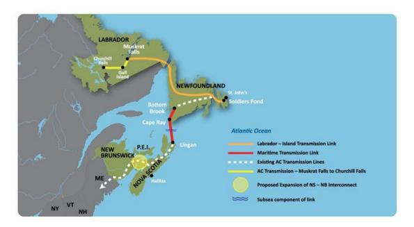
The Lower Churchill Generation Project's two (2) proposed installations, Gull Island and Muskrat Falls, will have a combined capacity of 3,074 MW and can provide sixteen point seven (16.7) terawatt hours of electricity per year. The proposed eleven hundred (1,100) kilometer high voltage direct current (HVdc) link will be the first of its kind in
