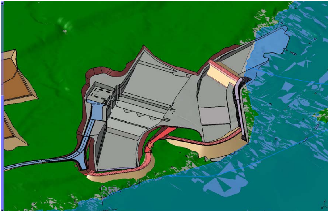
Figure 10-7 – Completion of Bulk Excavation (Powerhouse and Spillway) (shows early construction activity by main civil contractor)
