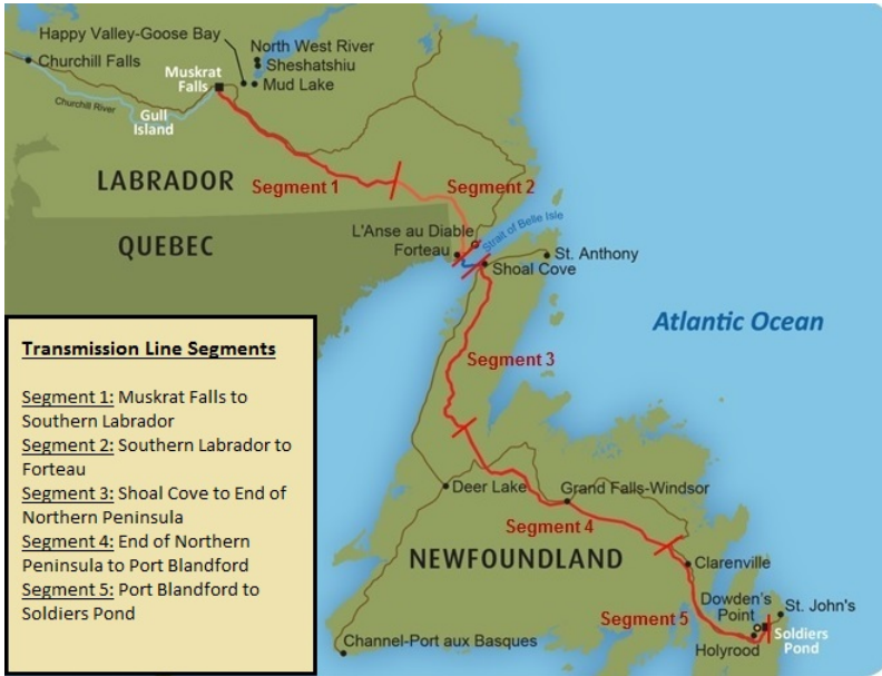
Figure showing the route for the Labrador-Island Transmission Link by Segment
