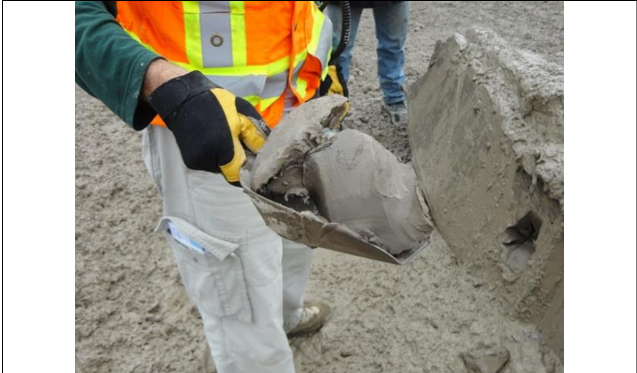
Photo E.17: Sample of cohesive, plastic "lower clay" from the base of the North Cutoff. (July 14, 2016)
