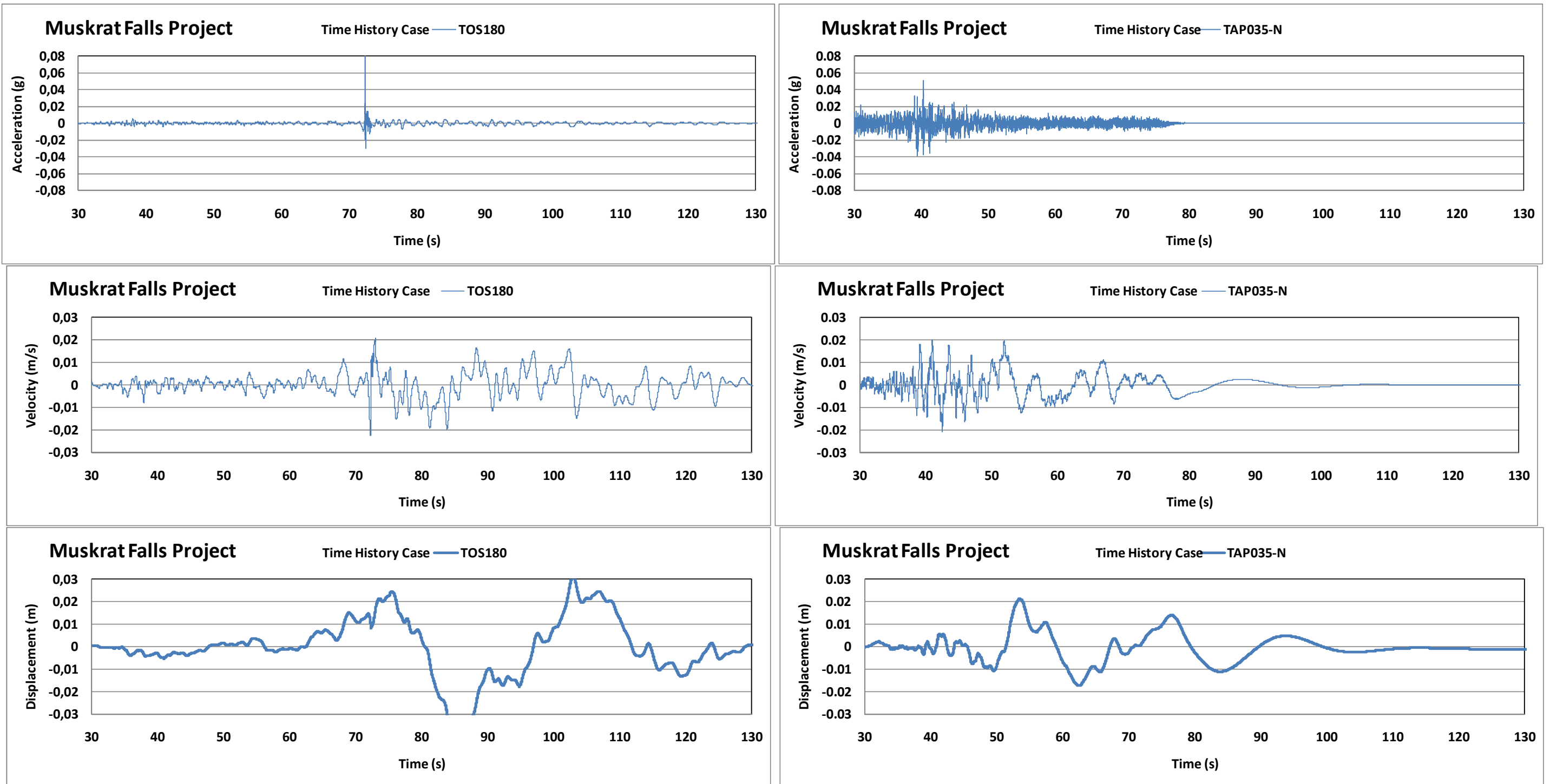
Figure E-2 – Spectral Matched Input Motions - Selection for 2D Analyses – Acceleration, Velocity and Displacement
