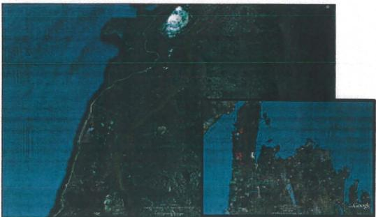
Zone 6 – Northern Peninsula Average Meteorological Loading Zone Maximum Ice: 50 mm (Glaze), Maximum Wind: 120 km/h, Combined Ice and Wind: 25 mm (Glaze) and 60 km/h
