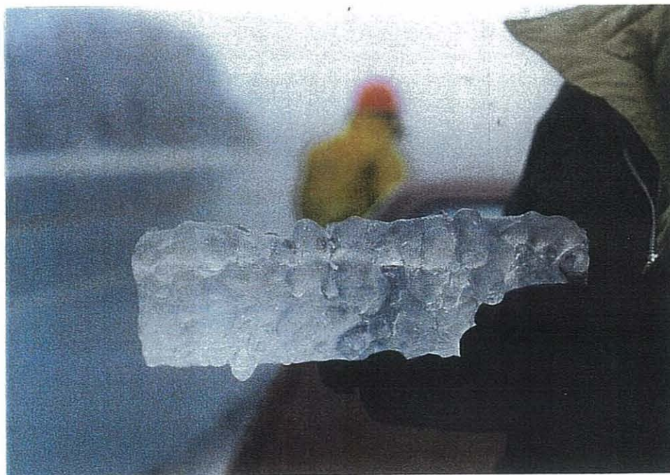
Photo No. 2-1 April 1984 Glaze Ice sample from Conductor-TL-237 ( weight 7.8 kg/m )
