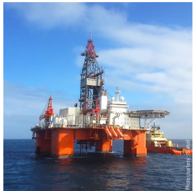
The semi-submersible West Aquarius is used for exploration, appraisal and development drilling in the province's offshore region.
